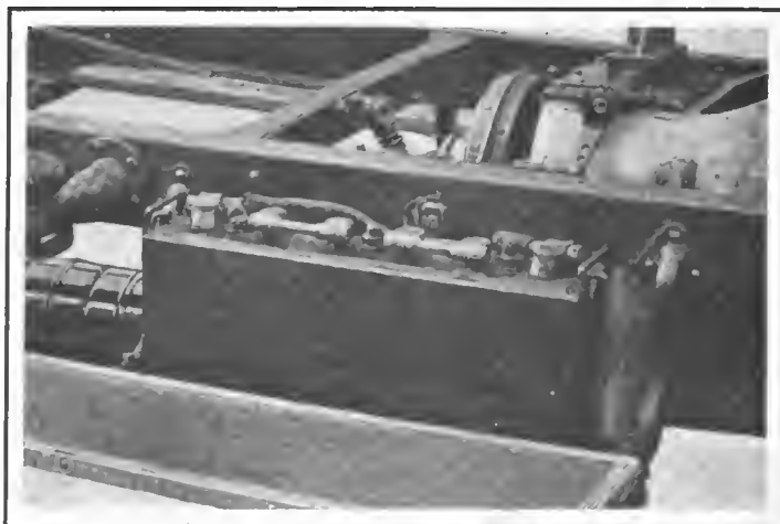
Neat disposition of the batteries on the Stearns-Knight new four. The three cells are placed in line, thereby permitting their suspension on the right between the frame and running board
